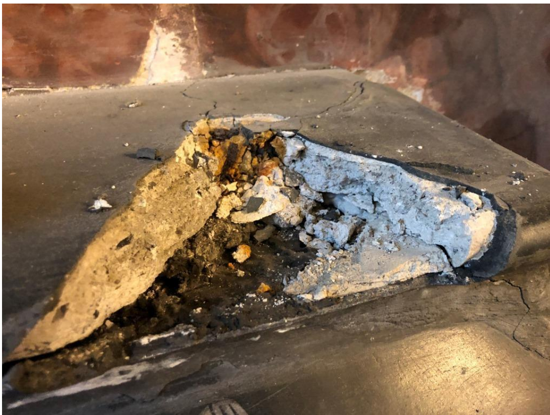
Plate 43: Detail of the top of the sarcophagus, right-hand side. A loose piece has been removed to show the construction of these panels with black scagliola over a coarse plaster base (not stone here), and the remains of one of three old iron fixing pins in the top. The expansion of the corroding iron can very clearly be seen to be the epicenter of structural disruption and cracking.
